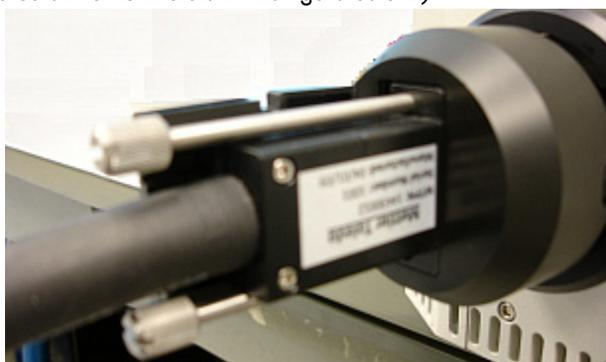
**Figure 7-7 DS Series optical interface with fiber installed**
