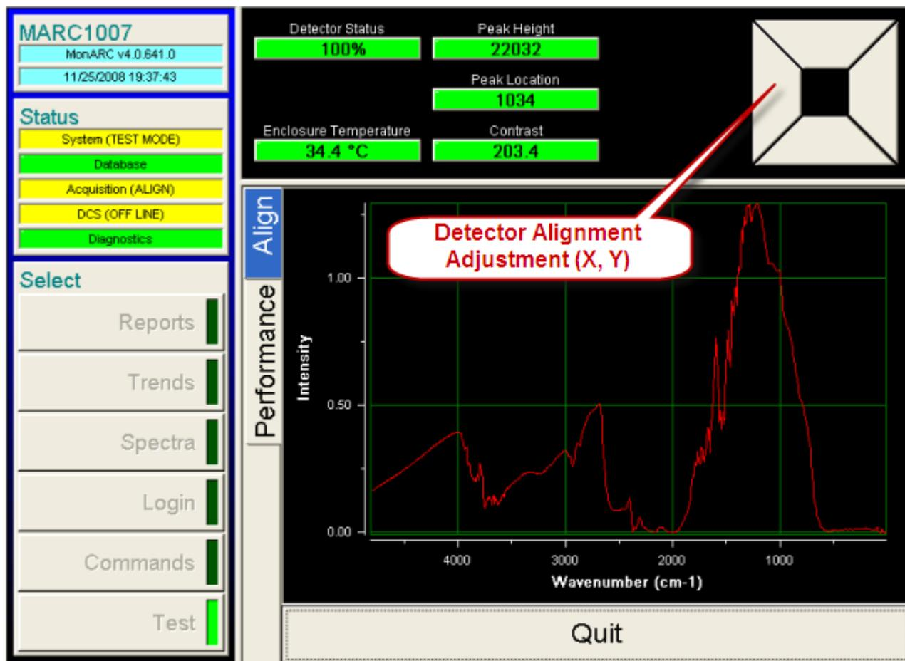
**Figure 8-8 Alignment in MonARC (Align tab)**
