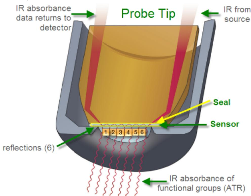
Figure 5-1 Sensor and seal at probe tip
