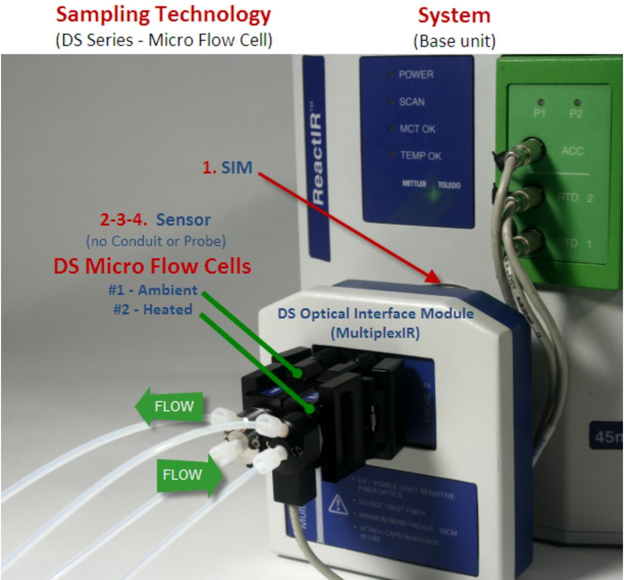
Figure 1-5 DS Micro Flow Cell sampling technology—(shown on a ReactIR 45m)
