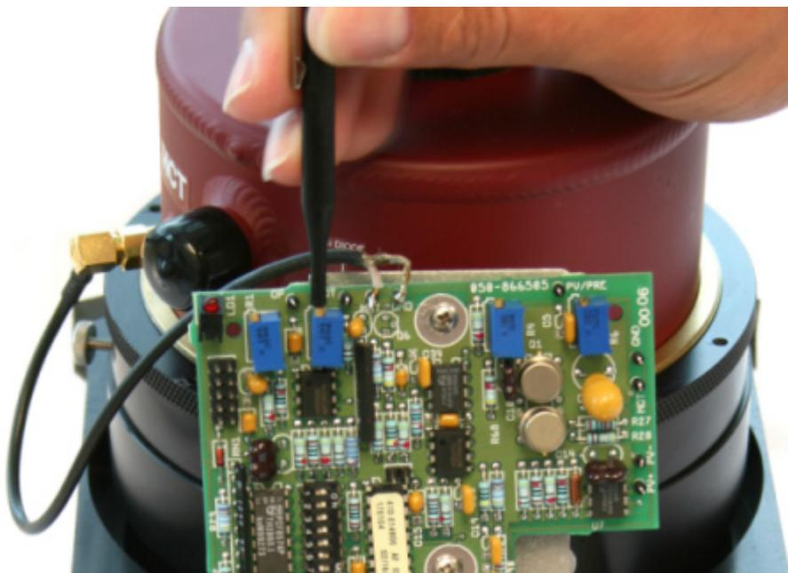
Figure 7-13 Gain pot adjustment on older model iC10 (with cover removed)
