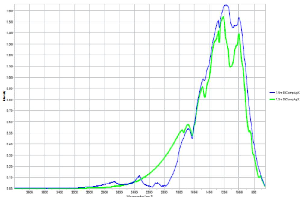
Figure 8-1 Single beam for DiComp (blue) and SiComp (green) 1.5m AgX FiberConduit
