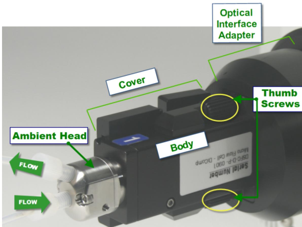
Figure 6-4 DS Micro Flow Cell (ambient)—Labeled
