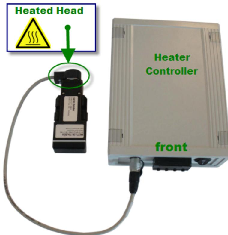
Figure 6-6 Heater connection to controller
