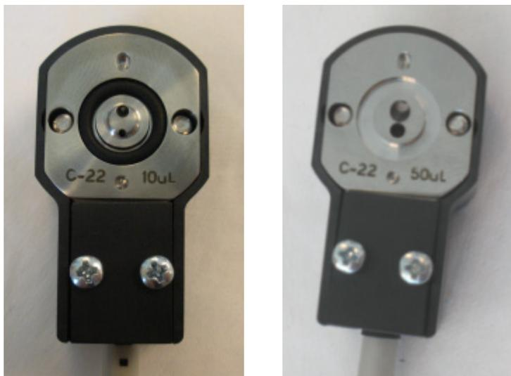
**Figure 6-5** Flow cell head internal volume—10 $\mu\text{L}$  (left) or 50 $\mu\text{L}$  (right)
