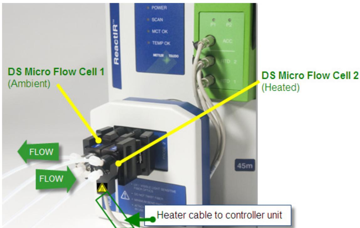
Figure 6-3 Two DS Micro Flow Cells on ReactIR 45m
