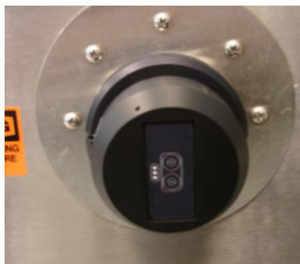
**Figure 2-7 DS Series Single Optical Interface Module installed on SIM**
