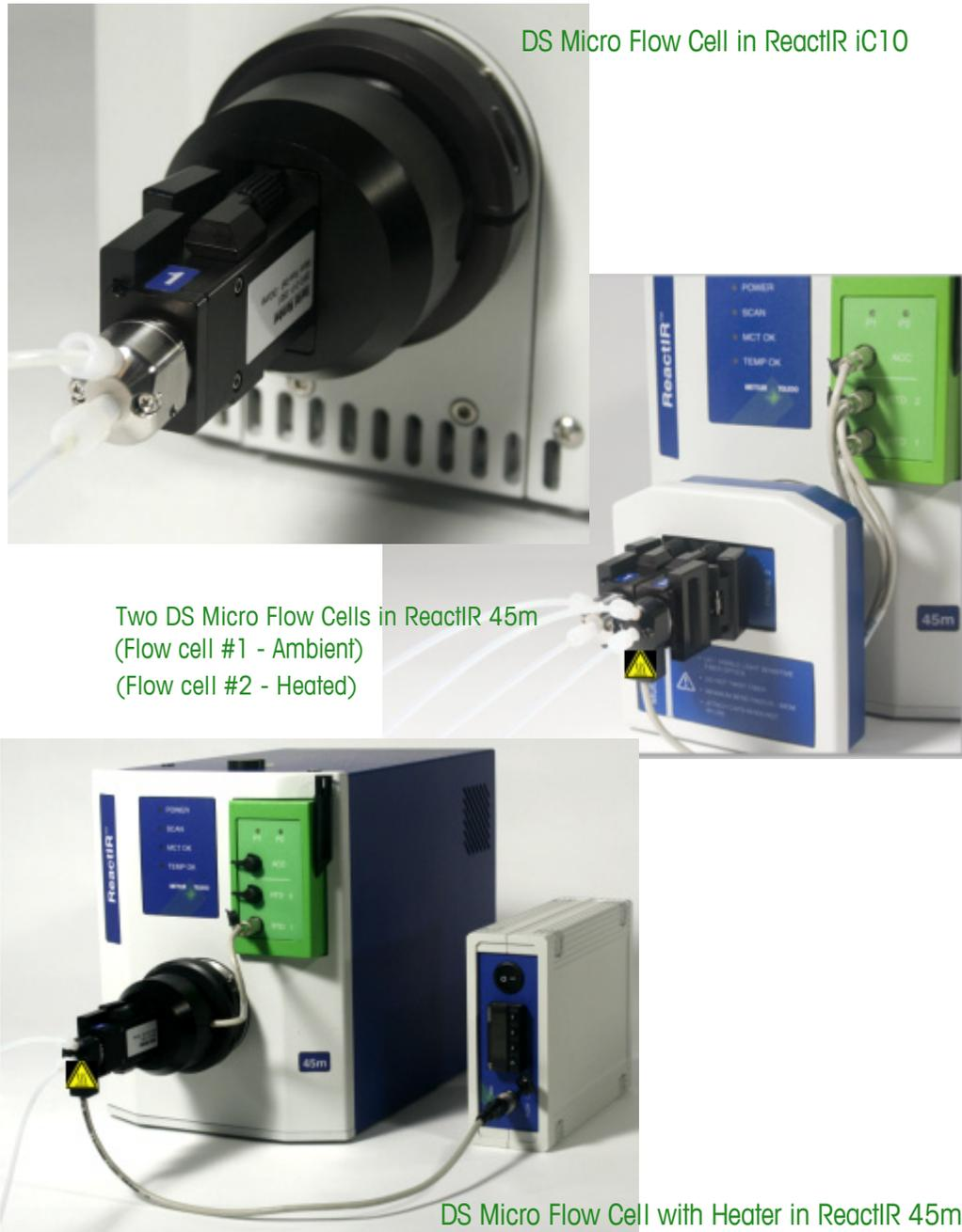
Figure 6-2 DS Micro Flow Cell examples
