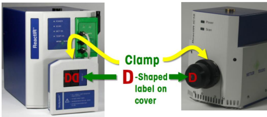
Figure 6-10 Multiplex (MUX) and Single Optical Interface Modules installed
