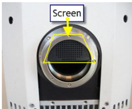
Figure 7-10 Energy compensation screen (in an iC10)
