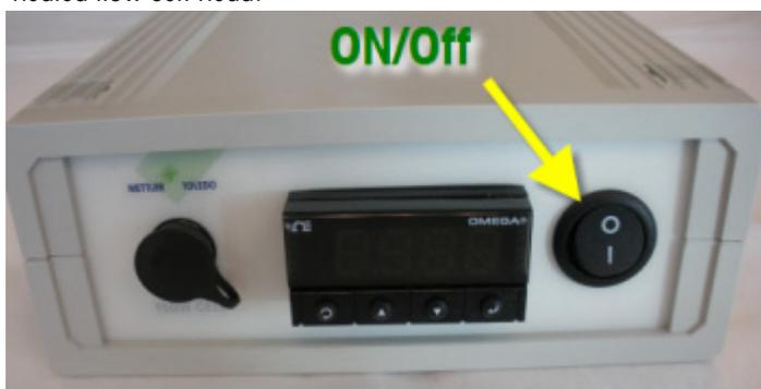
Figure 6-19 Heater controller front panel—Power
