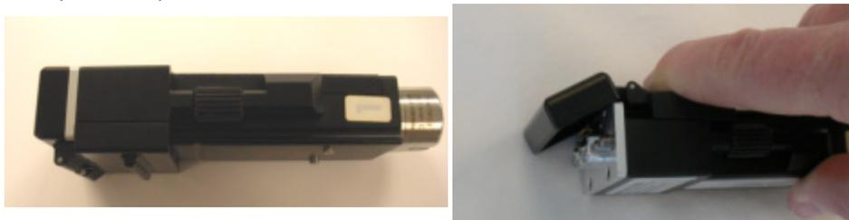
Figure 6-11 Protective cap before and during exposure of optics connection end
