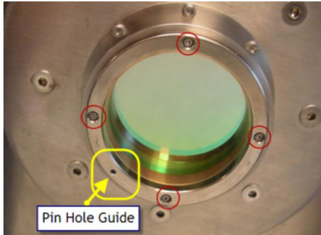
**Figure 7-4 DS Series interface retaining ring with pin hole guide**
