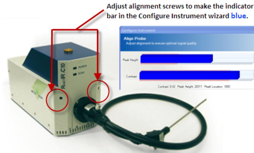
**Figure 8-7 Fiber Alignment on an iC10**
