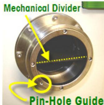
Figure 6-9 SIM showing mechanical divider and pin-hole guide
