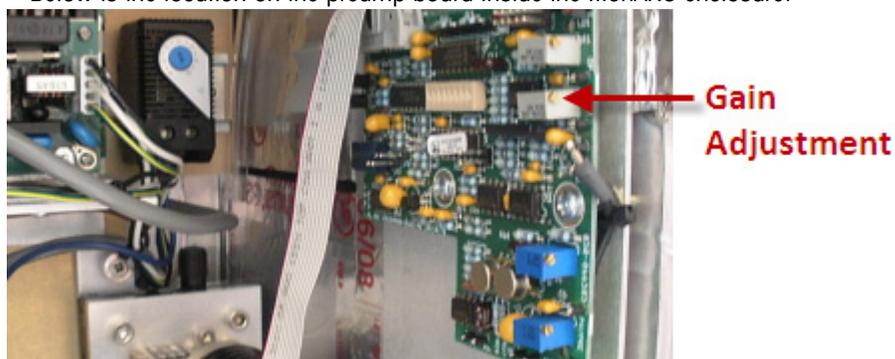
Figure 7-14 Gain pot adjustment on MonARC (requires open enclosure)
