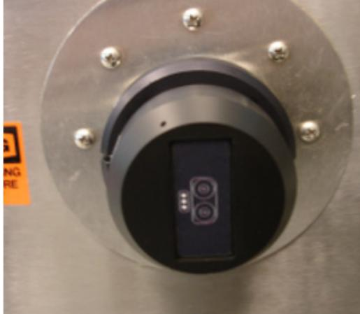
**Figure 7-5 DS Series optical interface on SIM flange**
