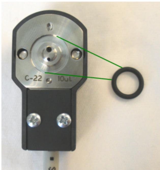
**Figure 6-21** O-ring in flow cell head—10 $\mu$ L (heated)
