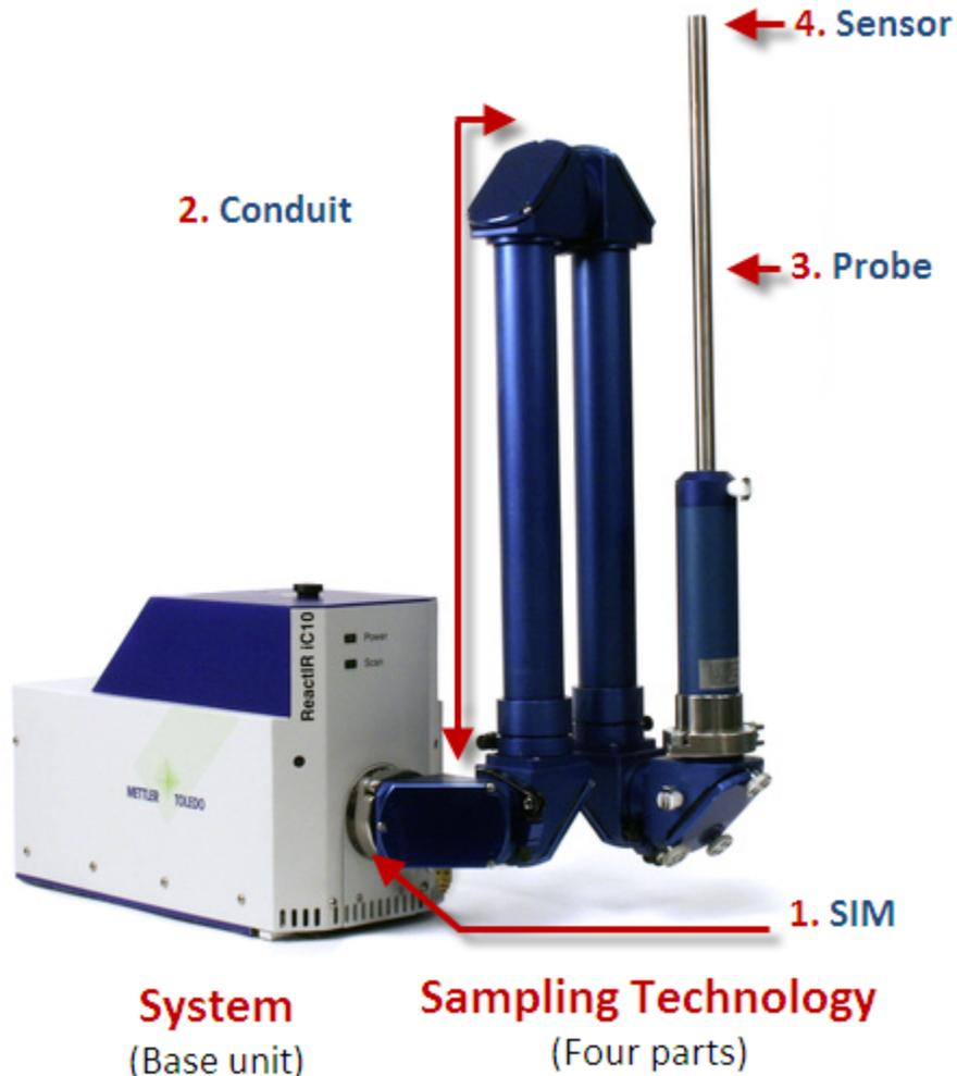
**Figure 1-1 Sampling technology—(mirror conduit and probe on a ReactIR iC10)**
