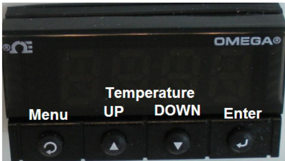
Figure 6-17 Temperature controller—setting buttons
