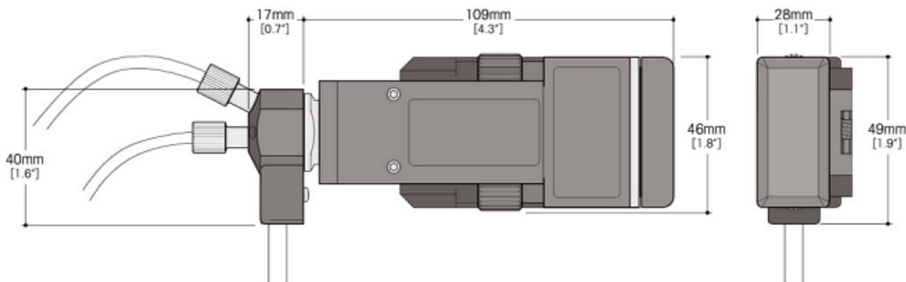
Figure 6-8 DS Micro Flow Cell—Dimensions
