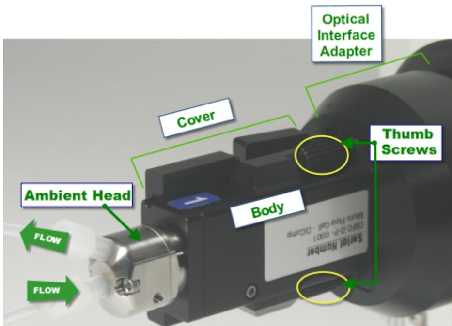
**Figure 6-12 DS Micro Flow Cell (ambient) installed in a SINGLE Optical Interface Module**
