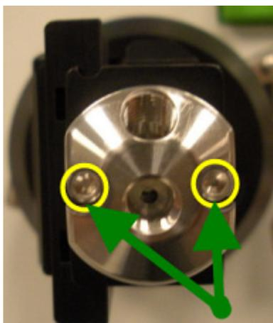
Figure 6-20 DS Micro Flow Cell head screws (shown on ambient model)
