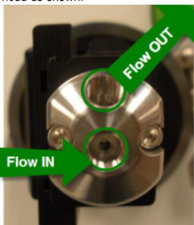
**Figure 6-16 Input and output to flow cell head (ambient)**
