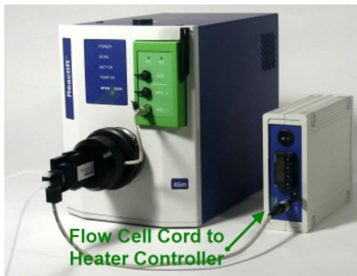
Figure 6-13 DS Micro Flow Cell (heated) connected to heater controller
