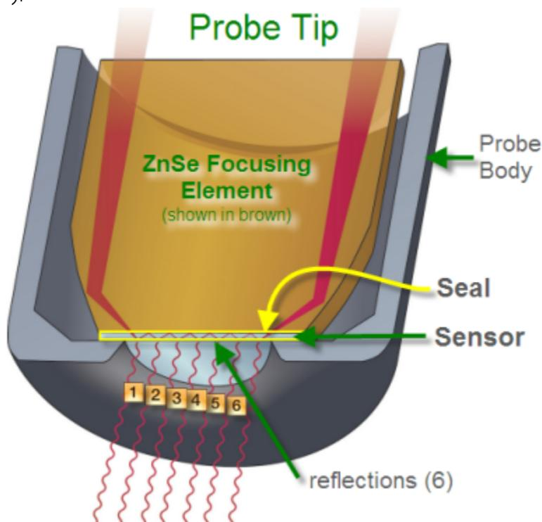
Figure 4-17 Diagram of probe tip
