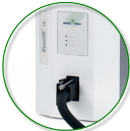
**Figure 7-9 DS Series FiberConduit installed on a ReactIR 15**
