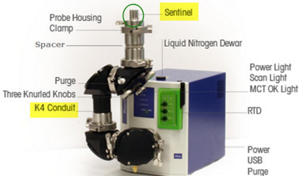
Figure 7-1 Sentinel (shown on a ReactIR 45m)
