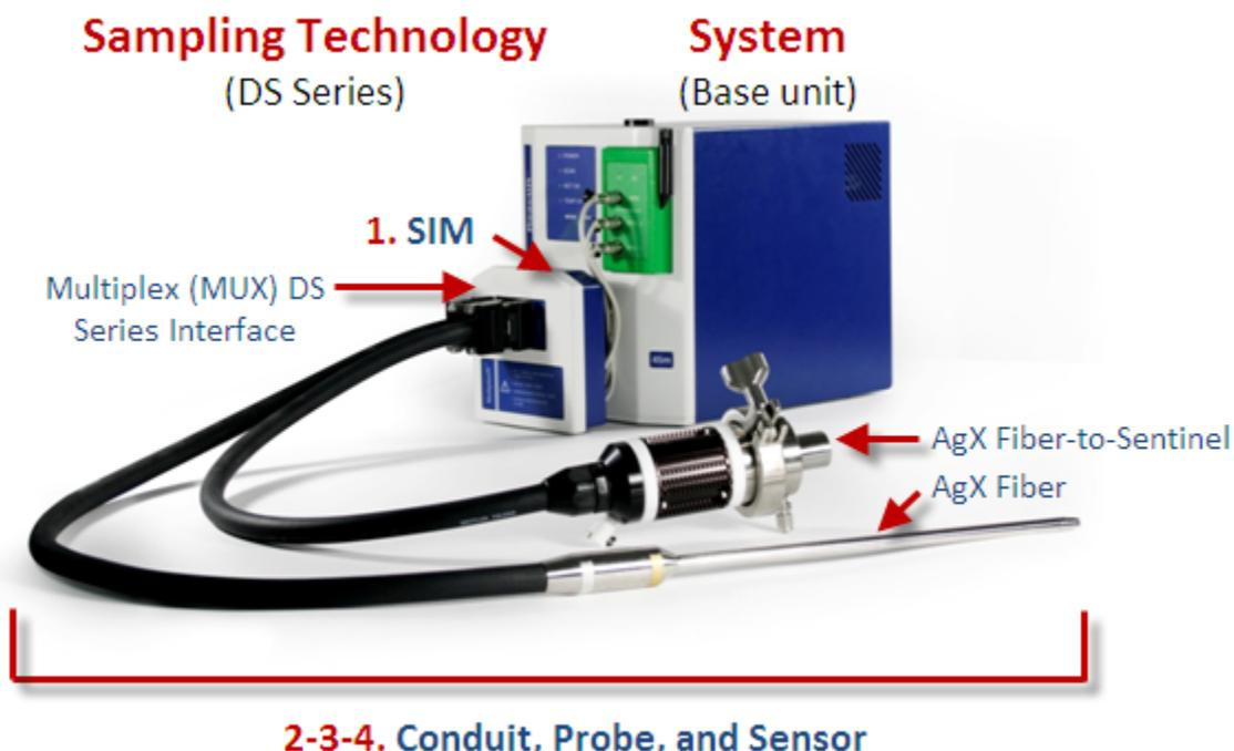
**Figure 1-2 DS Series sampling technology—(shown on a ReactIR 45m)**
