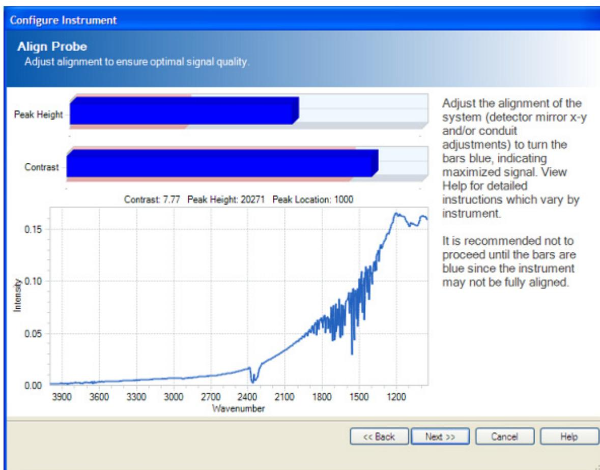
Figure 8-11 Probe alignment in iC IR software (Configure Instrument)
