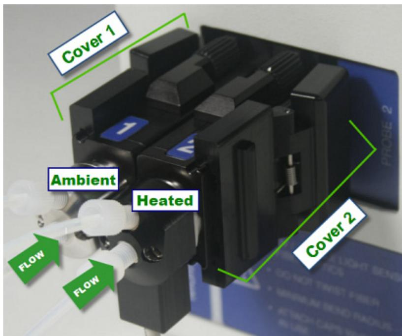
**Figure 6-18** Two flow cells (ambient on left, heated on right) in proper orientation
