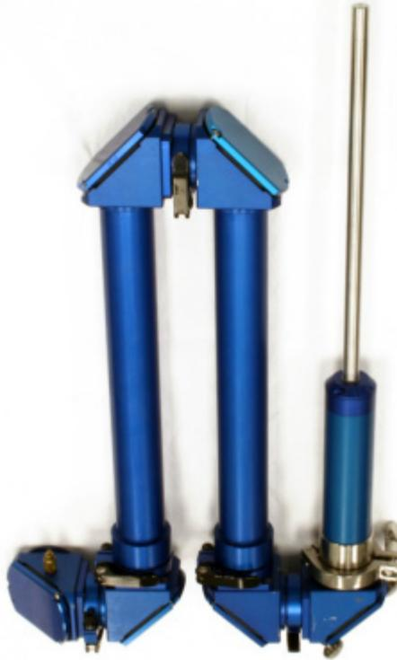
**Figure 3-14 K6 Conduit (with 16mm probe)**
