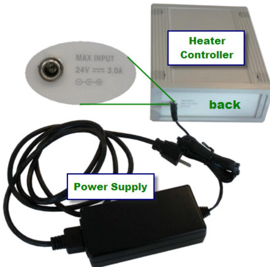
Figure 6-7 Heater controller power supply
