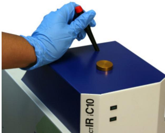
Figure 7-12 Gain pot adjustment on newer model iC10
