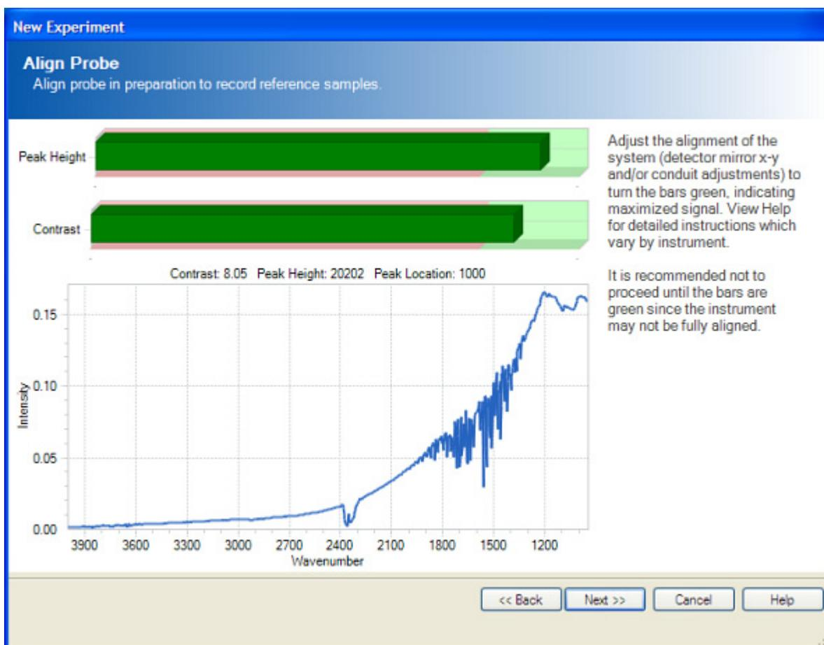
**Figure 8-10 Probe alignment in iC IR software (New Experiment)**
